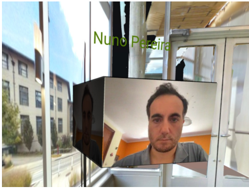
Figure 2: Example of how video can be texture mapped on avatars such that they are visible from multiple directions. Note that the front-facing face is lighter compared to the sides, providing a cue to where the user is facing. In the example, the user is inside a 3D scanned model of a real venue.
